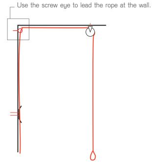
3. Hang the rope. Make sure the loop is underneith the pulley
